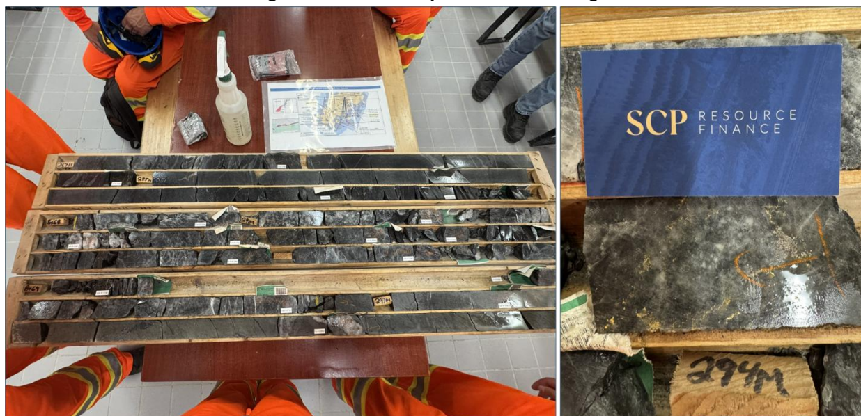
Figure 5. S Vein core photos and visible gold
