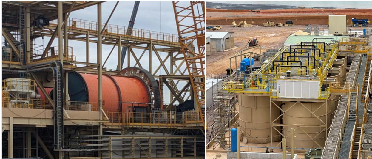
Figure 2. (A) Grinding mills assembly and (B) CIL circuit
